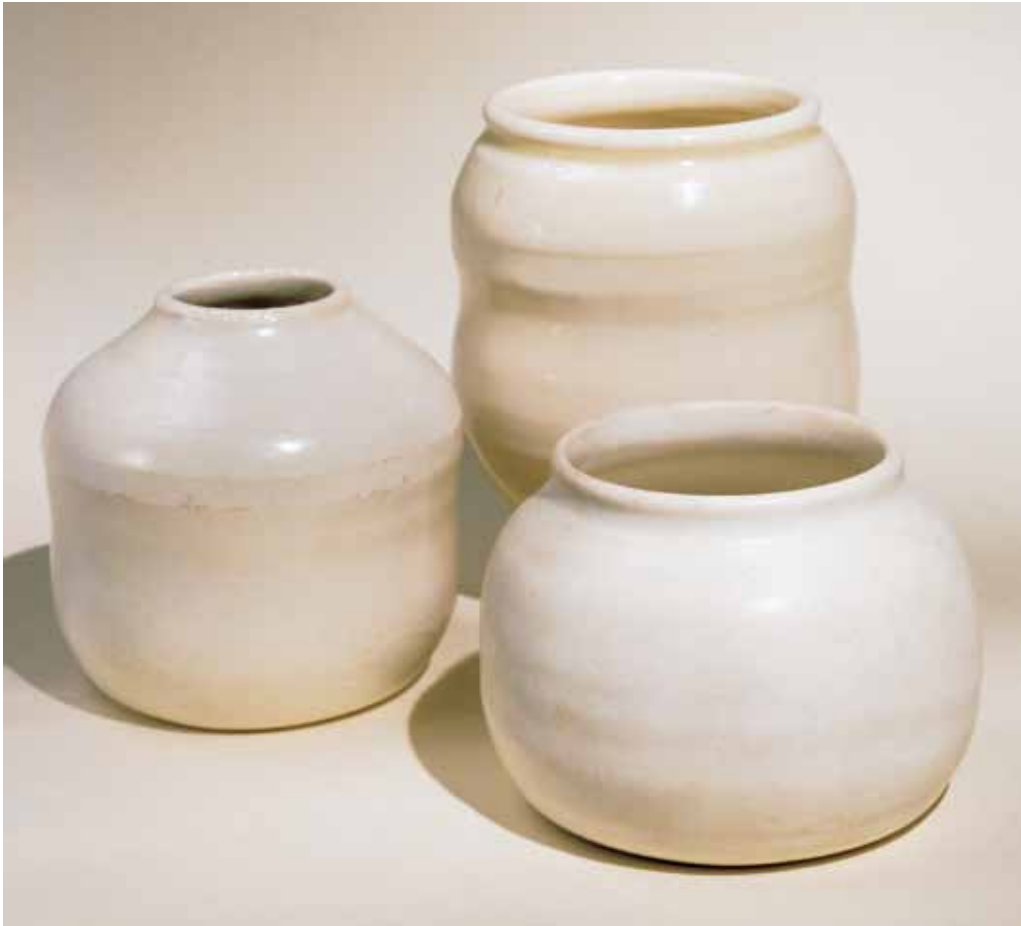
Cone 5–6 oxidation. Porcelain claybody. Left: Satin-matt surface: Nepheline Syenite 80%, Wollastonite 20%. Back: Gloss surface: Jacky’s Clear: Nepheline Syenite, 50; Colemanite, 10; Wollastonite, 10; Flint, 20; Zinc oxide, 5; Ball Clay, 5; Bentonite, 2. Front: Matt surface: Ron’s White Matt #5: F-4 Feldspar, 55; Whiting, 15; EPK, 16; Zinc oxide, 14.
