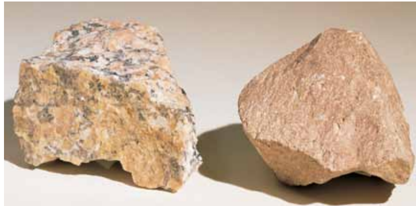
Left: Granite. Slow-cooled, coarse-grained, igneous rock containing 25% quartz, 50% feldspar (mostly potash in this sample), some muscovite, biotite, and/or amphibole.
