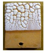
**Crazing** = Small hairline cracks in glazed surfaces that usually appear after firing but can appear years later. It is caused by a mismatch in the thermal expansions of glaze and body. A glaze of higher expansion shrinks more than the clay to which it is attached and therefore crazes.
