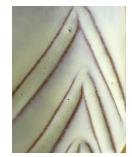
**Shivering (peeling)** = A defect in glazed ware where the glaze is compressed by a body having a higher thermal expansion. While it is normal, even necessary for glazes to be under some compression to avoid crazing and improve ware strength, over compression will actually cause the glaze to peel off the ware on edges to relieve the stress. Shivering is the opposite of crazing.
